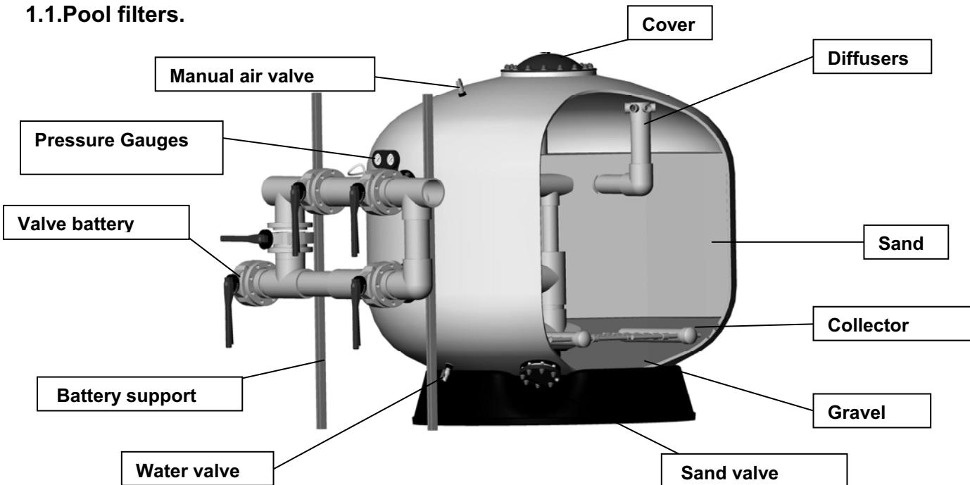
The filters are, without a doubt, the most important accessories for filtering water. And their object is to eliminate suspended materials and to clarify the water.
